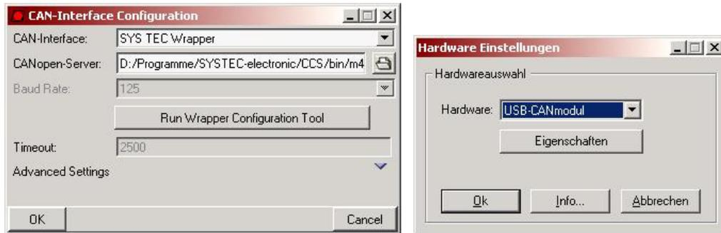
5. In the CDM select in the menu *Connection* → *Connect*. With this, the red LED at the USB-CANmodule should go out.
