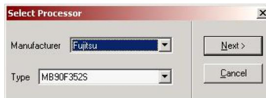
Confirm these setting with "Next >". In the next dialog you adjust the properties of the microcontroller. At that point please set the PLL factor to 6 and enter the requested transfer rate under "Speed":
