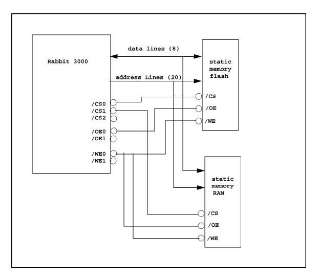
Figure 8-2. Typical Memory Chip Connection
