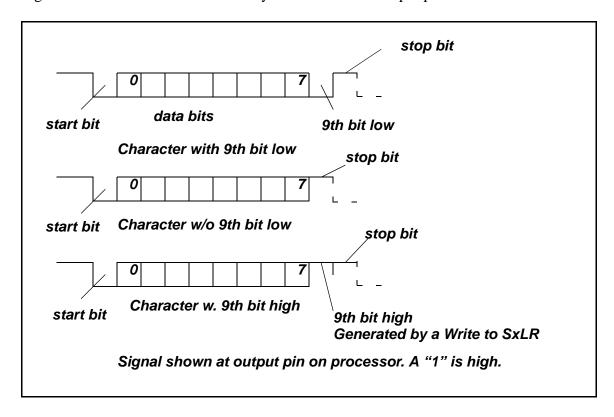
Figure 12-9. Asynchronous Serial Output Patterns
