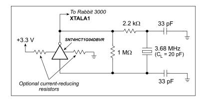
Figure 16-13. Reduced-Power External Main Oscillator
