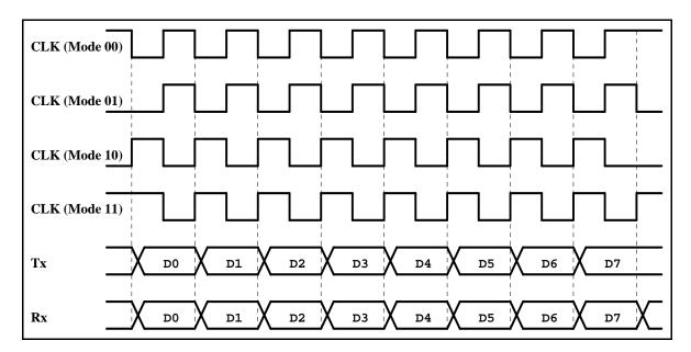
Figure 12-5. Clock Polarities Supported in Clocked Serial Mode
