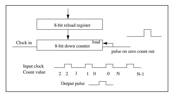
Figure 11-2. Reload Register Operation
