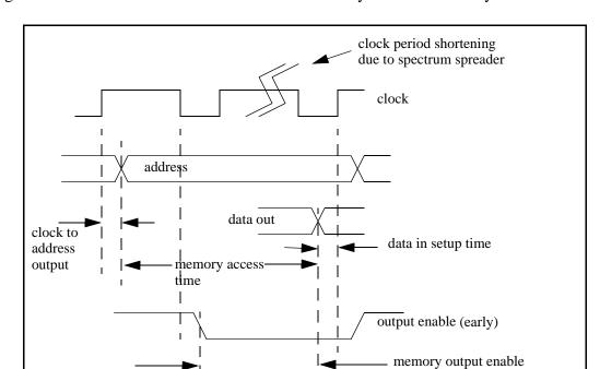
Figure 16-4 illustrates the sources that create memory access time delays.
