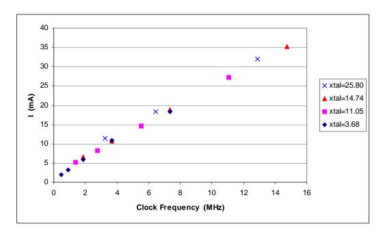
Figure 16-10. Rabbit 3000 System Current vs. Frequency at 3.3 V (enlarged view over 0–16 MHz range)
