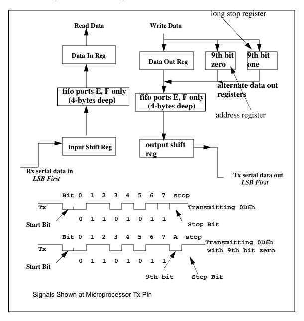
Figure 12-2. Functional Block Diagram of a Serial Port
