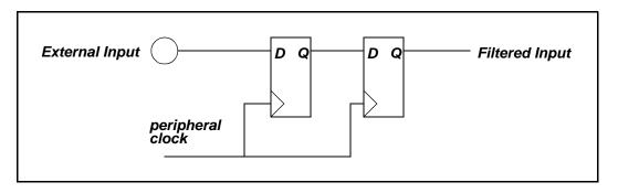
Figure 2-2. Digital Filtering Input Pins
