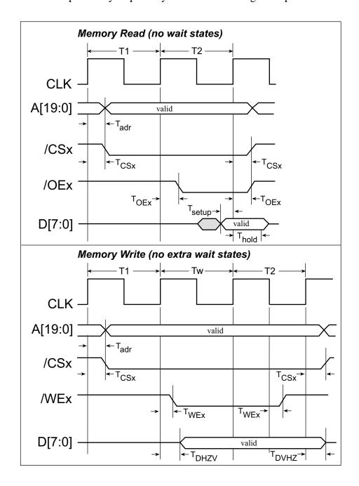
Figure 16-2. Memory Read and Write Cycles
