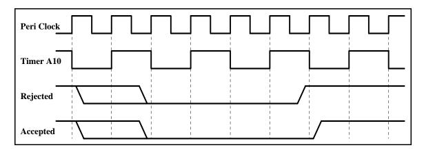
The Quadrature Decoder generates an interrupt when the counter increments from FFh to 00h or when the counter decrements from 00h to FFh. The timing for the interrupt is shown below. Note that the status bits in the QDCSR are set coincident with the interrupt, and the interrupt (and status bits) are cleared by reading the QDCSR.
