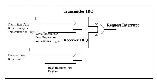
Figure 12-3. Generation of Serial Port Interrupts
