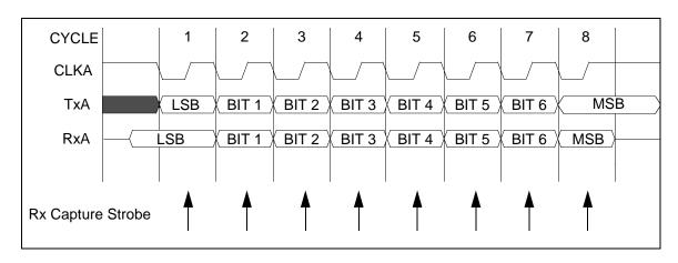
Figure 12-6. Full-Duplex Clocked Serial Timing Diagram with Internal Clock (Mode 00)
