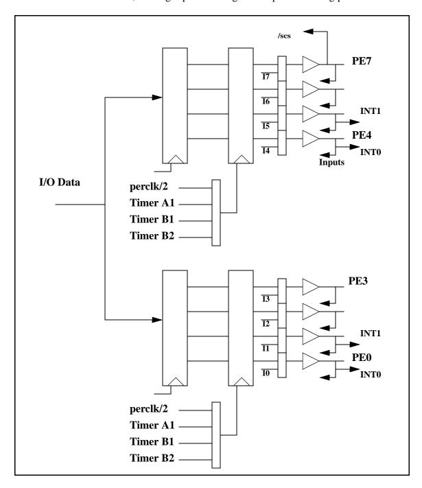
Figure 9-2. Parallel Port E Block Diagram
