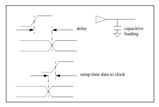
Figure 16-1. Parameters Used to Describe Memory Access Time
