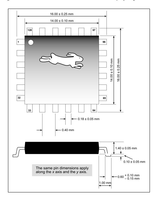
Figure 5-2. Mechanical Dimensions Rabbit LQFP Package
