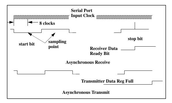
Figure 12-4. Serial Port Synchronization
