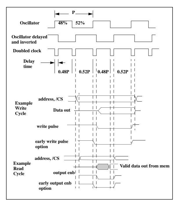
Figure 16-7. Clock Doubler and Memory Timing
