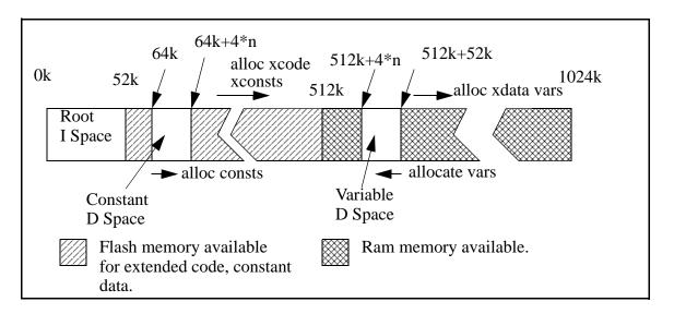
Figure 8-6. Use of Physical Memory Separate I & D Space Model
