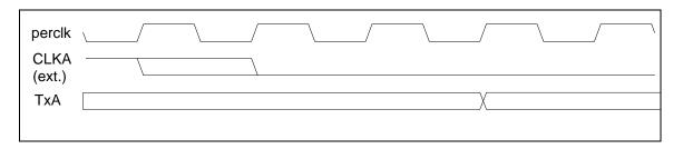
Figure 12-7. Synchronous Serial Data Transmit Timing with External Clock (Mode 00)
