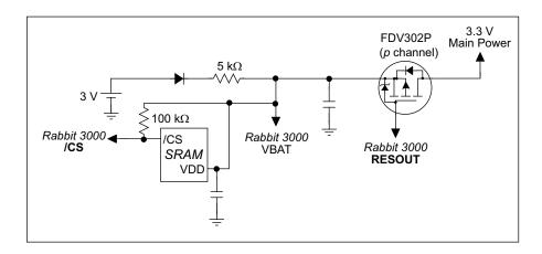
Figure 8-1. Battery-Backup Circuit
