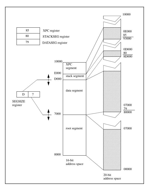
Figure 3-3. Example of Memory Mapping Operation
