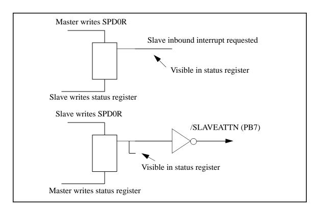
Figure 13-3. Slave Port Handshaking and Interrupts
