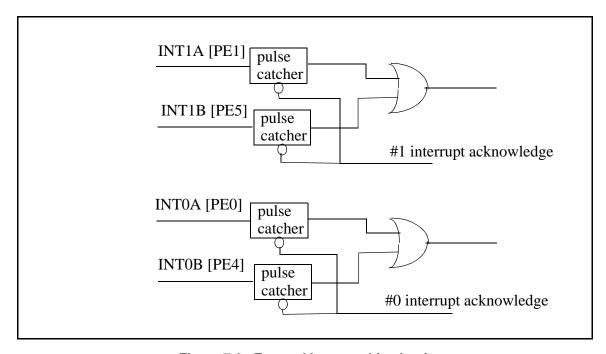
Figure 7-6. External Interrupt Line Logic
