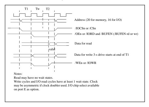
Figure 5-7. Bus Timing Read and Write
