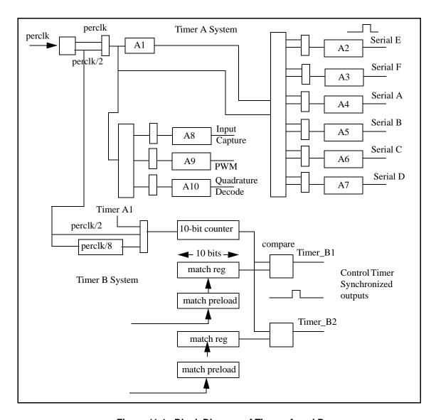
Figure 11-1. Block Diagram of Timers A and B
