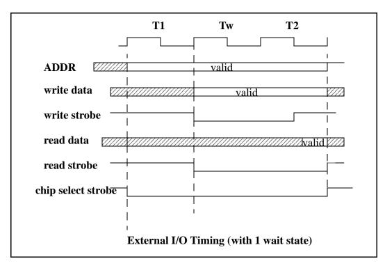
Figure 10-1. External I/O Bus Cycles
