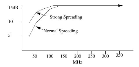
Figure 15-1. Peak Spectral Amplitude Reduction from Spectrum Spreader
