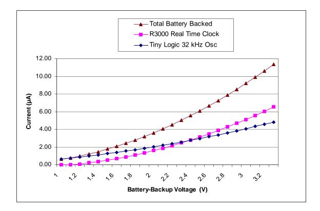
Figure 16-12. Current Consumption—Real-Time Clock and 32 kHz Oscillator Circuit
