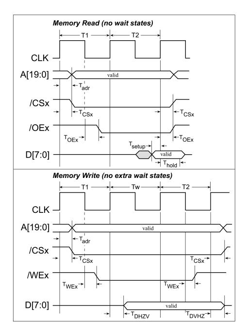
Figure 16-3. Memory Read and Write Cycles—Early Output Enable and Write Enable Timing
