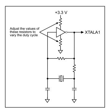
Figure 16-8. External Oscillator Buffer
