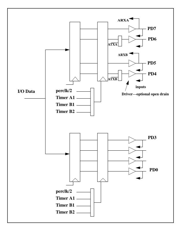
Figure 9-1. Parallel Port D Block Diagram
