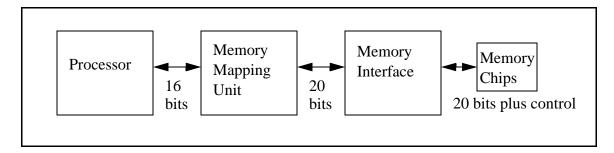
Figure 3-2. Addressing Memory Components
