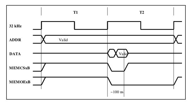
Figure 7-5. Self-Timed Chip Select Memory Read Cycle
