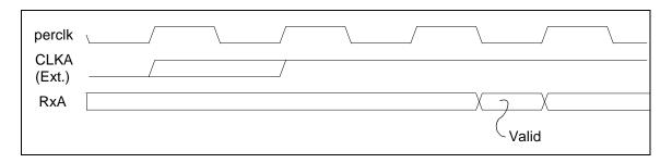
Figure 12-8. Synchronous Serial Data Receive Timing with External Clock (Mode 00)
