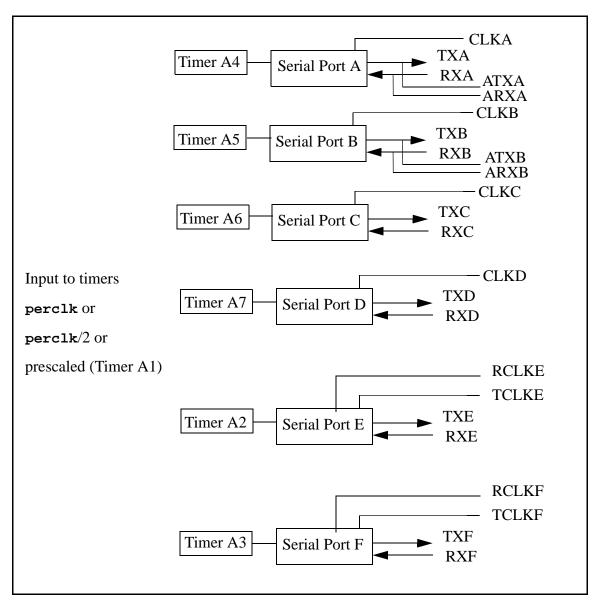
Figure 12-1. Block Diagram of Rabbit Serial Ports
