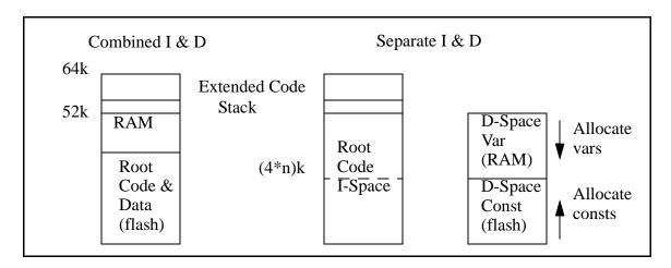
Figure 8-5. Combined versus Separate I & D Space
