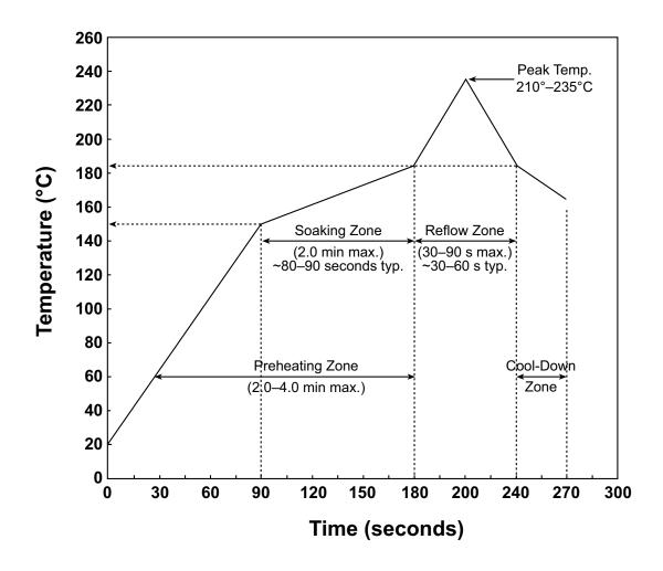
Figure 5-6. TFBGA Reflow Temperature Profile
