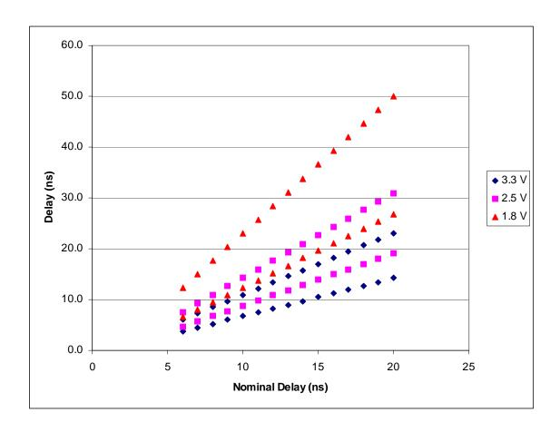
Figure 16-5. Clock Doubler Max-Min Clock Low Times
