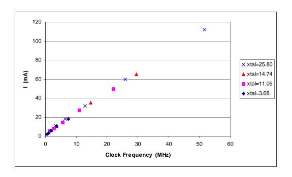
Figure 16-9. Rabbit 3000 System Current vs. Frequency at 3.3 V
