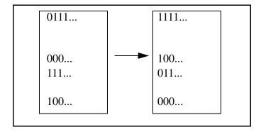
Figure 3-8. Mapping Signed Integers to Unsigned Integers by Inverting Bit 15
