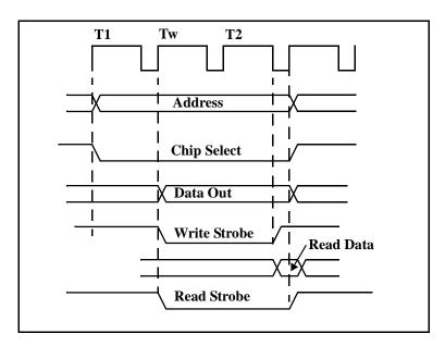
Figure 1. I/O Cycle Timing (no extra wait states)
