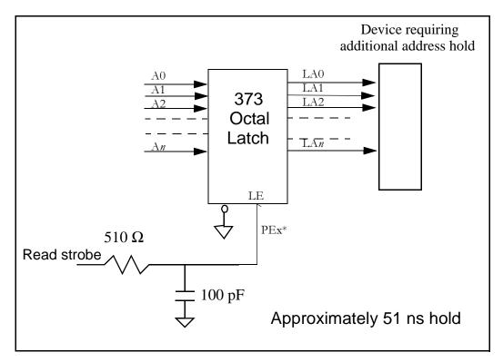
Figure 2. Address Hold Using a Transparent Latch
