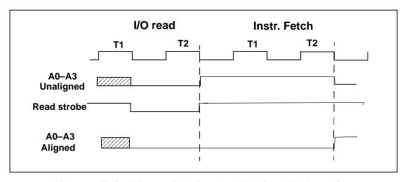
Figure 3. Timing Diagram for Aligned and Unaligned Address Lines
