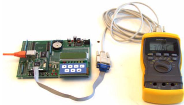
Let's figure out how to do this. First, we need a processor with both a serial port and an Ethernet port to use as our serial-to-Ethernet bridge. Luckily something like the RCM3000 will do nicely. Simply plug it into a development board, which will provide it with regulated power and RS-232 level conversion, and we are almost ready to go...except the software of course.
