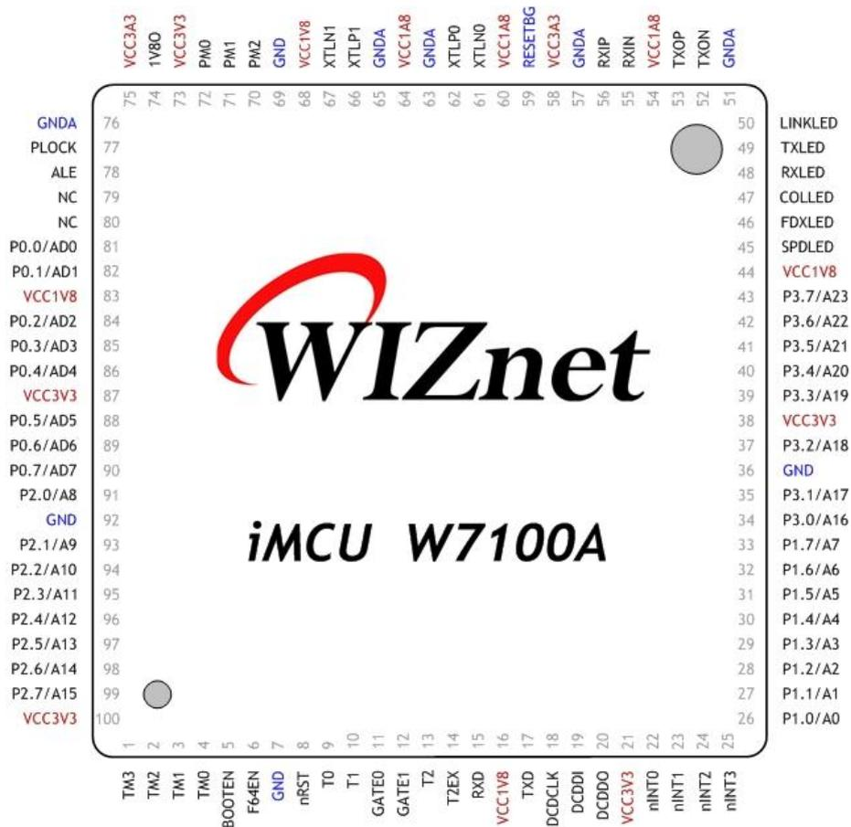
Fig 1. W7100A 100pin LQFP package
