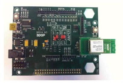
Figure 7: DR1174 Carrier Board (with a JN516x Module)
