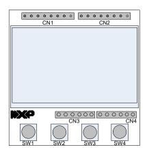
Figure 16: DR1201 LCD Expansion Board Layout
