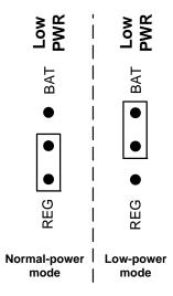
Figure 10: Lower-Power Mode Selection (using Low PWR Jumper)
