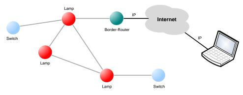
Figure 3: Wireless Network with IP Connectivity
