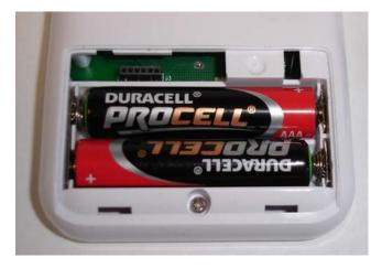
2. Insert the Programming Dongle onto the header in the battery compartment, as illustrated below.
