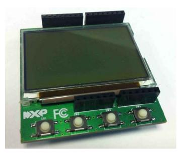
Figure 17: DR1201 LCD Expansion Board
