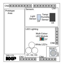
Figure 12: DR1175 Lighting/Sensor Expansion Board Layout
