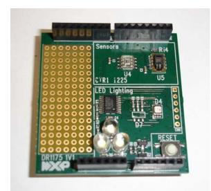
Figure 13: DR1175 Lighting/Sensor Expansion Board
