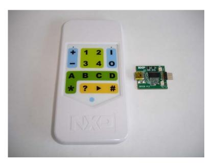
Figure 5: DR1159 Remote Control Unit (and DR1128 Programming Dongle)
