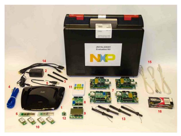
Figure 4: JN516x-EK001 Evaluation Kit Components
