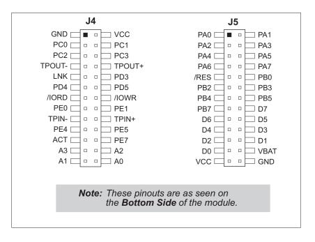
Figure 1. RCM2200 Connector Pinout
