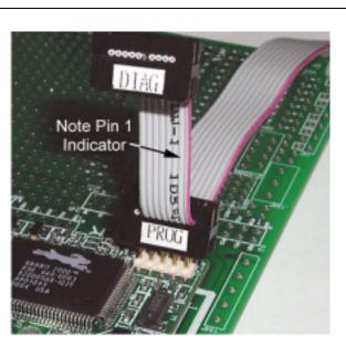
Figure 5. Connect Programming Cable to RCM2200
