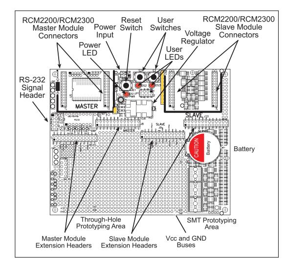
The Prototyping Board is shown below in Figure 2, with its main features identified.
