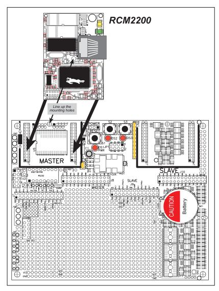
Figure 4. Installing the RCM2200 on the Prototyping Board
